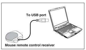
The remote control may fail to operate if the mouse remote control receiver is exposed to bright sunlight or fluorescent lighting. In such a case, change position or direction of the mouse remote control receiver and retry.
